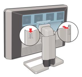
**2** Slide the cover upwards while holding the clips pressed.
